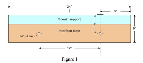
Interface plate material – 5-ply  $\frac{1}{2}$  inch plywood or  $\frac{3}{4}$  inch hardwood.
